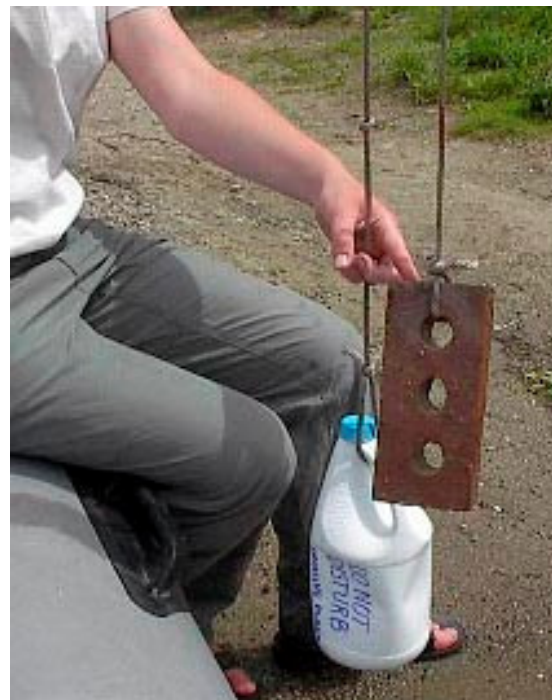
Homemade buoy marker using cored brick and empty, thoroughly rinsed plastic jug
